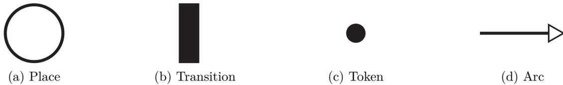
Figure 7 – Components of a Petri Net.
