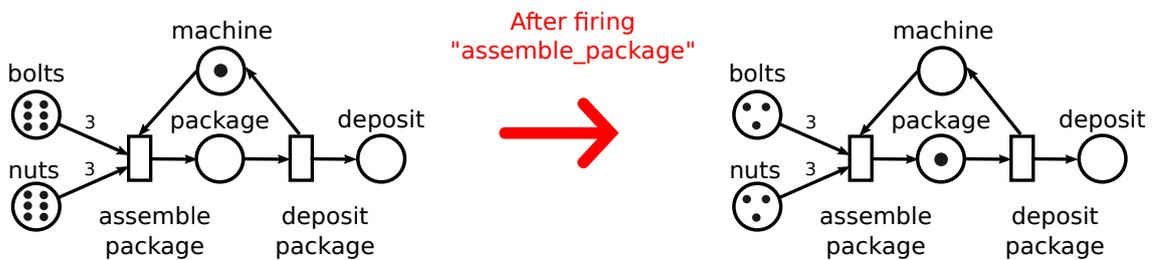
Figure 11 – Firing of a transition - example
