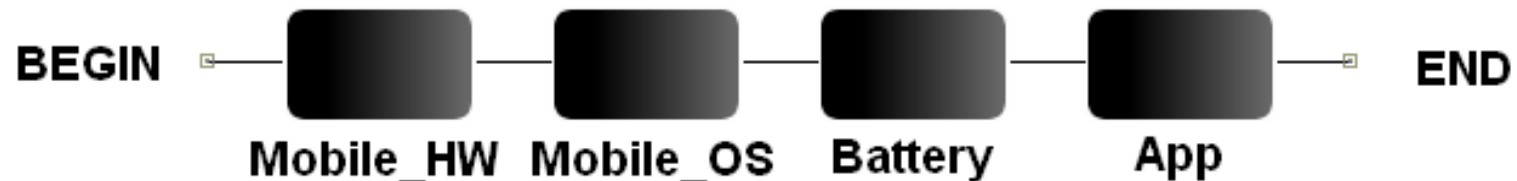
RBD model for the non-redundant mobile device
