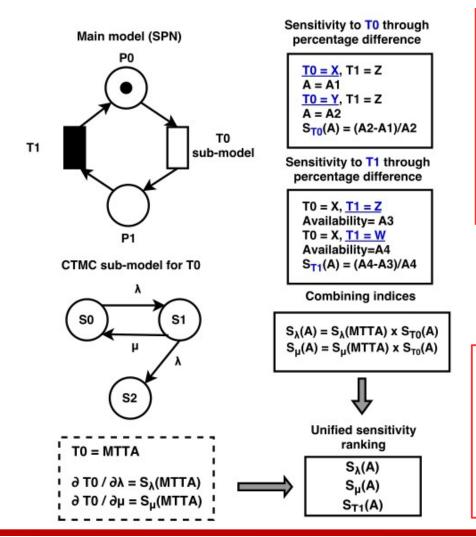
When the SPN can only be solved through **simulation**, the indices from CTMC sub-models are multiplied by indices of corresponding SPN transitions. Therefore, we follow the **chain rule**:
